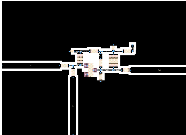
Figure 19. Finished Layout for Mixer Circuit
