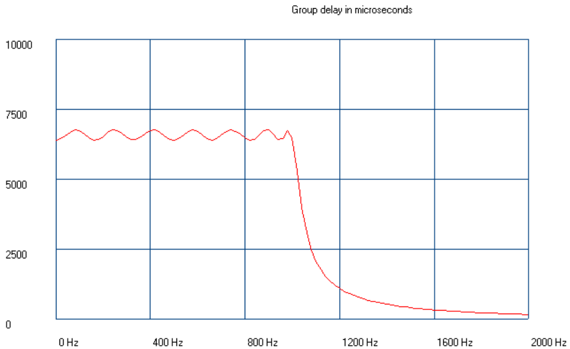
Group delay equalization of 7 th order Tchebyscheff lowpass.
